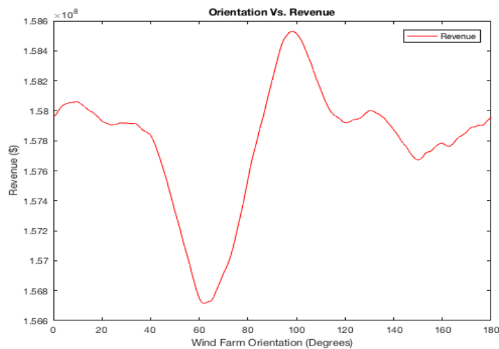
Figure C.11: Total revenue values for each orientation of the 9X4 rectangular wind farm with 4D and 8D spacing.
