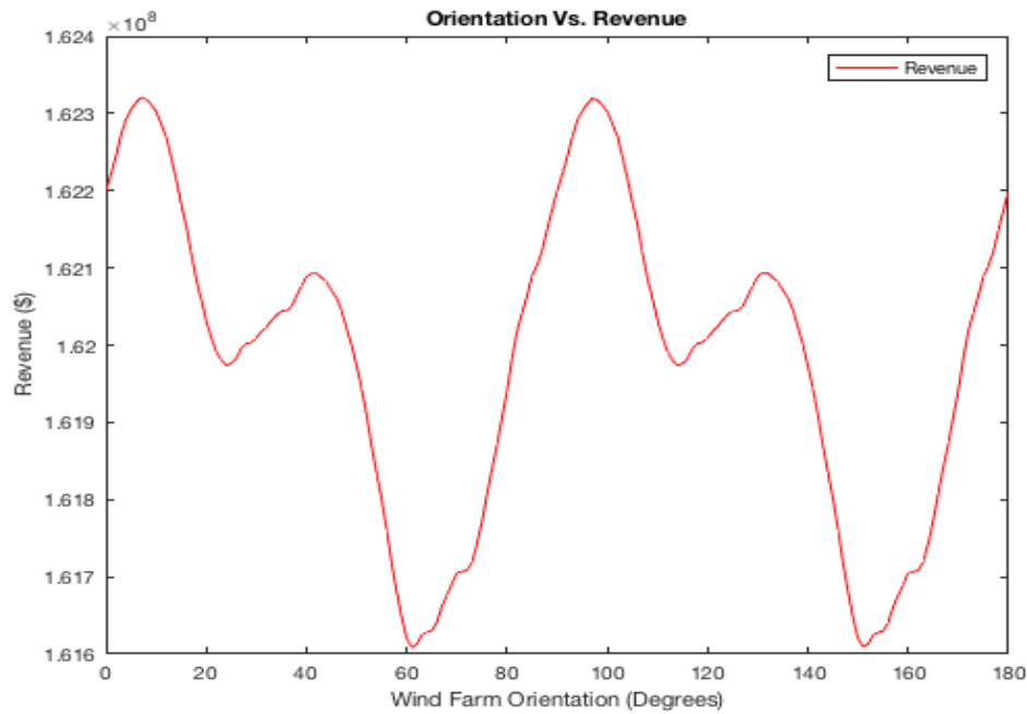
Figure C.19: Total revenue values for each orientation of the 6X6 square wind farm with 8D spacing.
